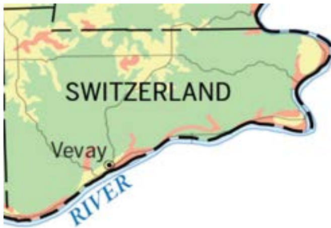
Figure 22 Earthquake Liquefaction Potential Map
